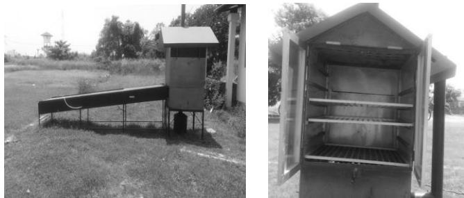
Figure 7. Solar dehydrator used to dry low-salted fish
